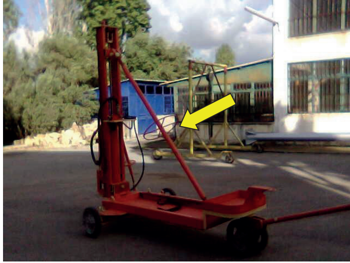
This arm is used for keeping the boom vertical
